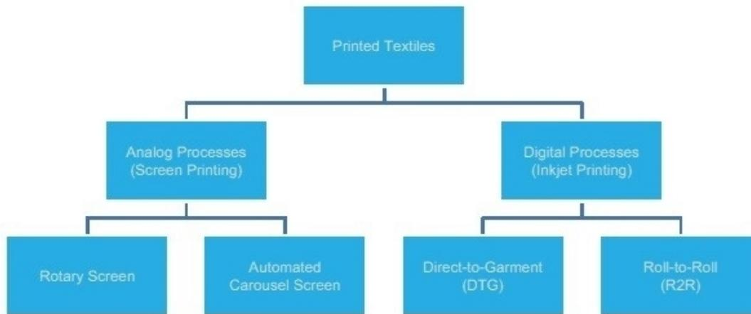
Screen printing is the most commonly used printing process for textiles. The two primary methods of screen printing are rotary screen printing and automated carousel screen printing.
