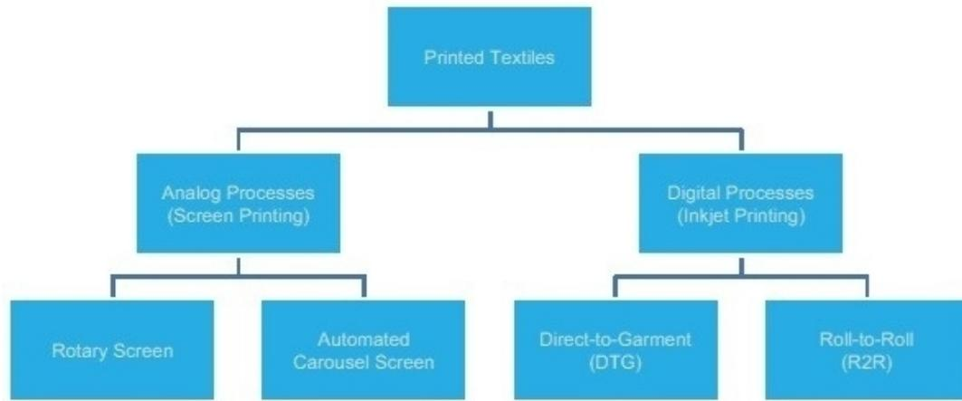
Screen printing is the most commonly used printing process for textiles. The two primary methods of screen printing are rotary screen printing and automated carousel screen printing.
